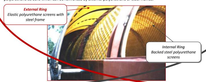
Besides our experience and ability in designing and manufacturing efficient screening surfaces is coupled by our engineering of the whole trommel structure for the hardest screening applications.
